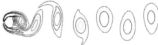
Fig. 14. Vorticity contour of the flow around a circular cylinder at Re = 200 .
